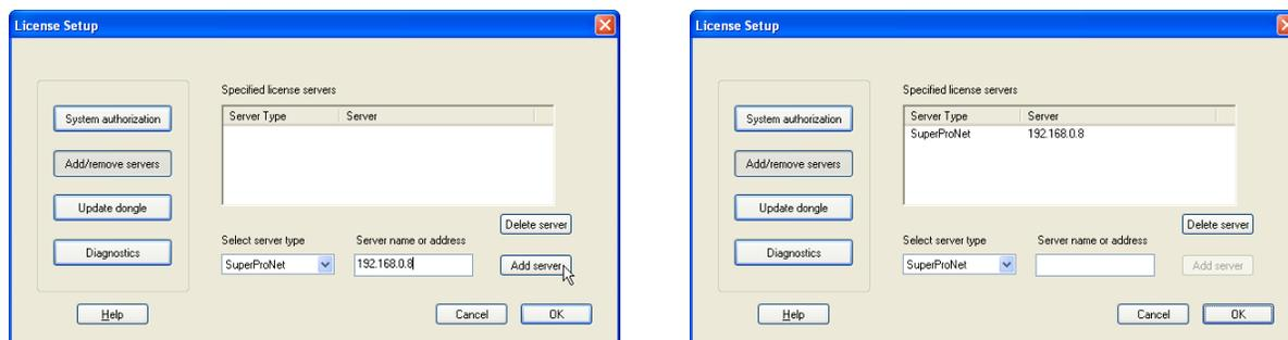
Entering the server's IP address (left) and viewing the server information (right) in the dialog box.
