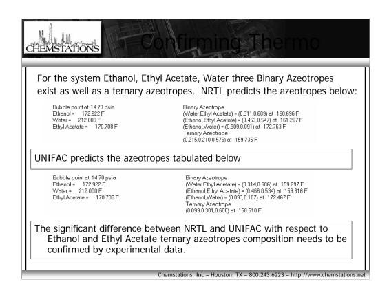
For the previous system two activity coefficient methods predicted the binary azeotropes but deviate in the analysis of the Ternary
