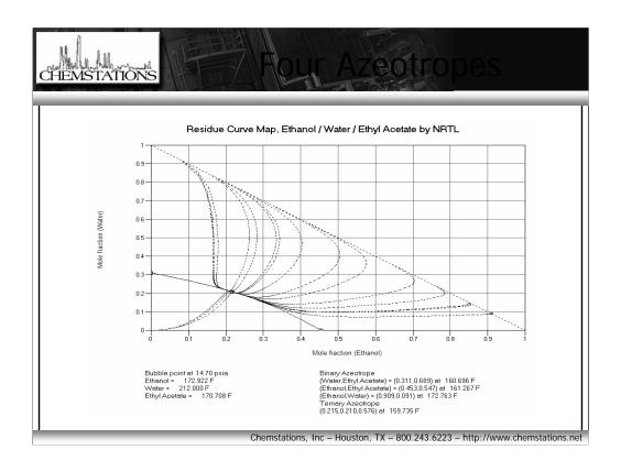
Residue Curve Maps can find ternary azeotropes (and in the case above 3 binary azeotropes)
