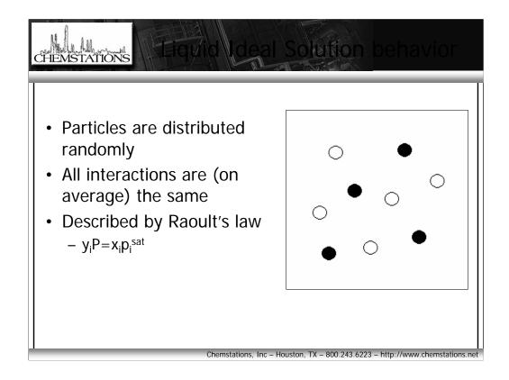
Most Thermodynamiv Vapor Liquid Equilibrium models are driven by the behavior of the molecules in the liquid phase
